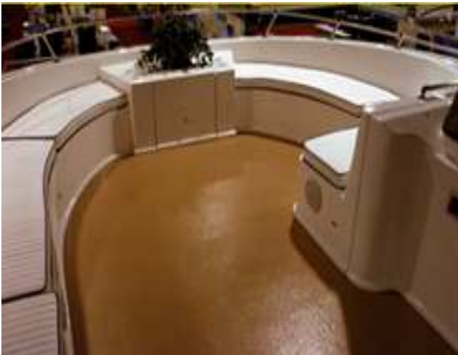
Yacht rear deck flooring using Coathylene® as a anti-slip agent
